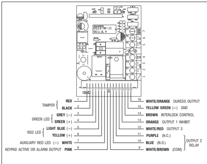
The connection facilities consist one set of terminal block mainly for Output 1 for door lock open; and one set of wire harness for Output 2 and 3, and the auxiliary functions.
