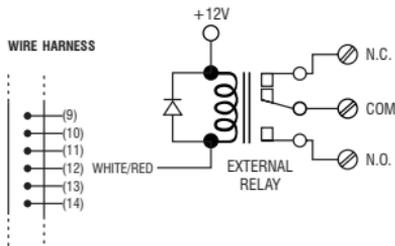
Output 3 is an open collector output prepared for auxiliary controls. It may be used for arm-disarm of a security system, enable and disable of a keypad or a protection zone etc.; it can also drive a relay to give full function of N.C. and N.O. outputs as like the output 2 making the keypad a ture 3 output system.
