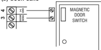
With the help of a Normally Closed door position sensor (usually a magnetic door switch) on the door to set up the following functions:
