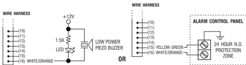
The DUESS Output will switch to (-) ground when duress code is entered. You may use it to turn ON an LED lamp and/or a small buzzer to notify a guard; or connect it to a 24 hour Normally Open protection zone of an alarm system.
