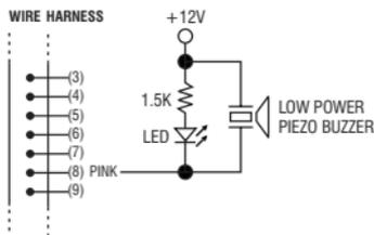
The Key Active Output will switch to (-) ground for 10 seconds whenever a key is touched. You may use it to turn ON an LED lamp and /or a small buzzer to notify a guard; or to energize a relay to switch ON lights or trigger an CCTV Camera to start recording.
